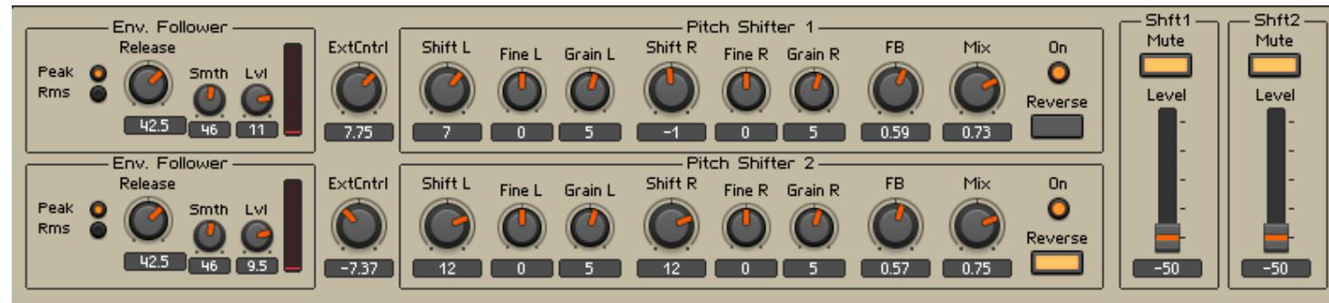
Control panel for an instrument implementing two stereo pitch shifters controlled by envelope followers. Two such instruments could be used to process the four instruments in a string quartet independently. Players may develop other methods.
